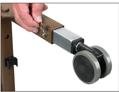
a. The four large pins are used if the height of the bed is to be locked at a set height. Set the height of the bed so that the hole in the leg is aligned with the hole in the bed end outer leg. Insert the pin through each of the four legs and install the spring clip on each.
